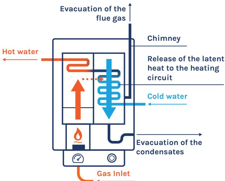
Schematic illustration of a gas condensing boiler
