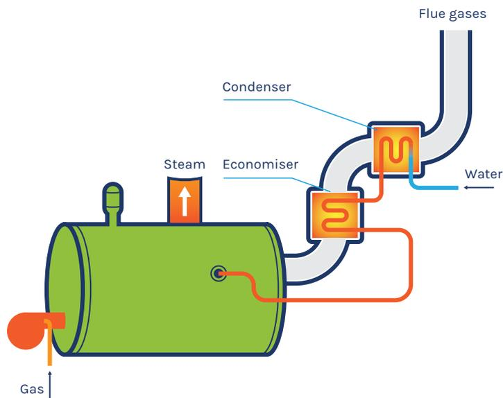
Schematic illustration of a couple economiser/condenser installed on a steam boiler (preheat of boiler feed water mode)
