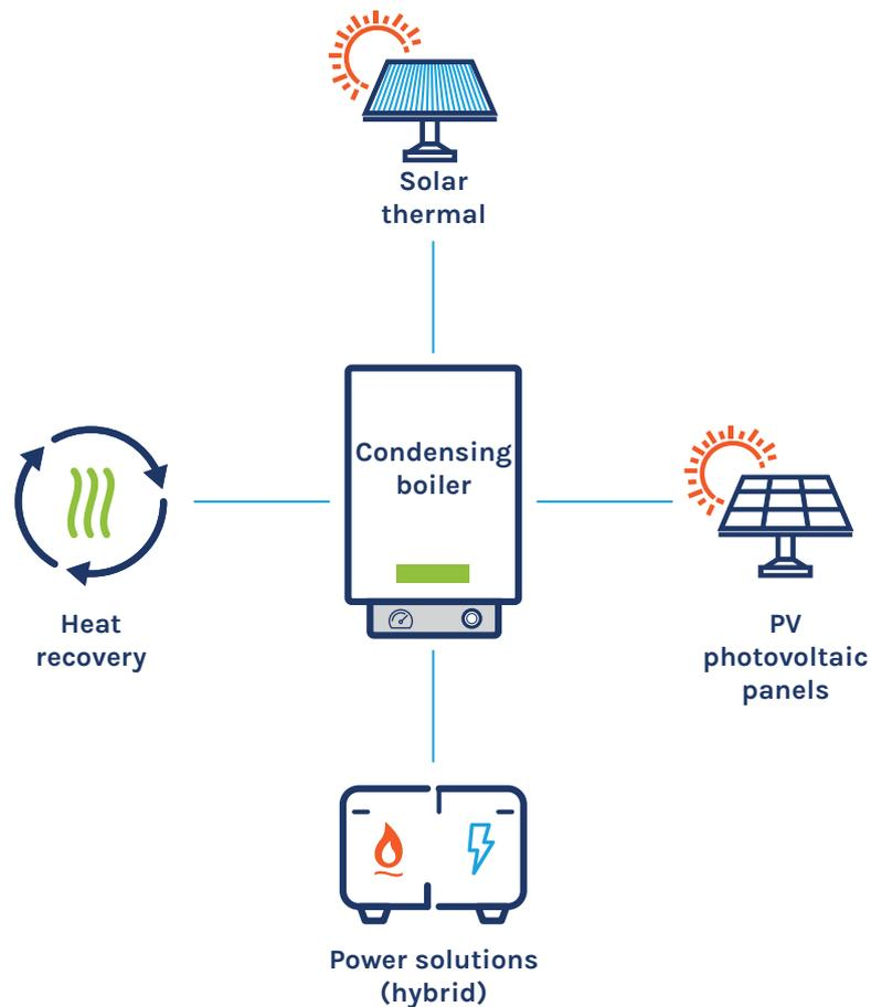
A condensing boiler can be coupled with one or more solutions
