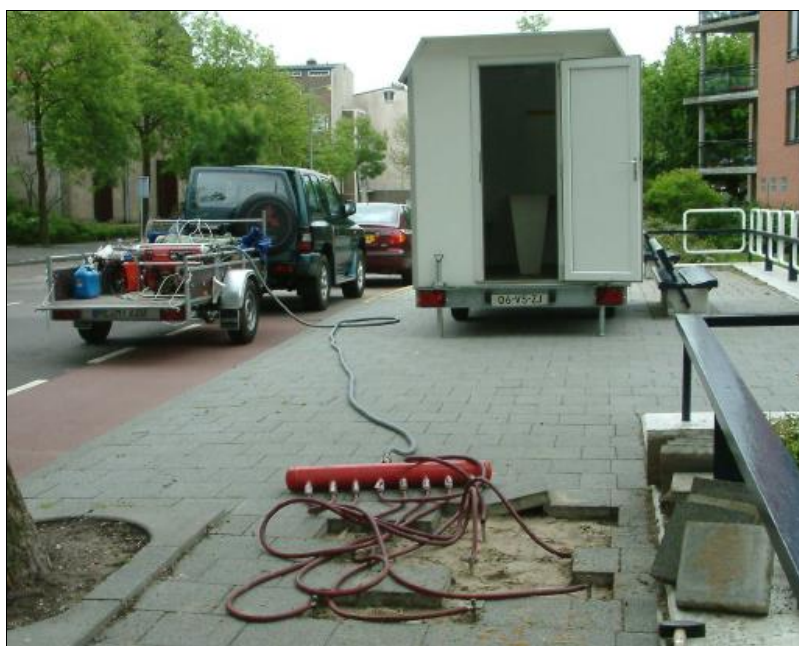
Figure 10-2: Emission rate measurement with suction method in Amsterdam
