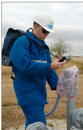
Figure 10-4: High Flow Sampler measurement on a facility
