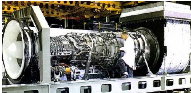
Photo 4: Gas turbine as compressor drive
